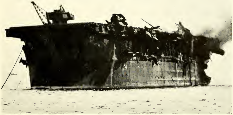
The light carrier INDEPENDENCE, located between 1000 feet and \frac{1}{2} mile from the projected Zeropoint, shows severe damage. Her 600 foot flight deck is broken in several places. Part of the deck planking has burned. Her four stacks have been demolished, and her antenna masts are bent or broken.
