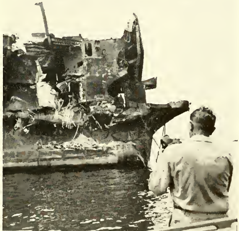
The light carrier INDEPENDENCE, located between 1000 feet and \frac{1}{2} mile from the projected Zeropoint, shows severe damage. Her 600 foot flight deck is broken in several places. Part of the deck planking has burned. Her four stacks have been demolished, and her antenna masts are bent or broken.
