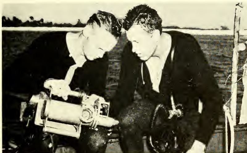
Dr. V. E. Brock (right) and Ensign Richard Cron, Navy diver, examine a camera specially designed for use underwater, as in photographing damaged portions of sunken ships. This work was made difficult after Test B by the potential dangers from radioactivity in the water or in the ships themselves.
