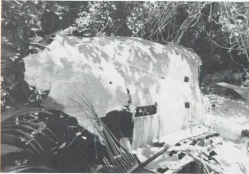
Fig. 11.42. Looking forward at wing root and fuselage. Bullet holes visible below two small square openings. (NPS photo by Kevin Foster)
