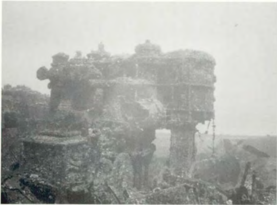
Fig. 9.15. SHOUN MARU's triple-expansion steam engine sits upright in its original location. (Photo by Mark Michael)
