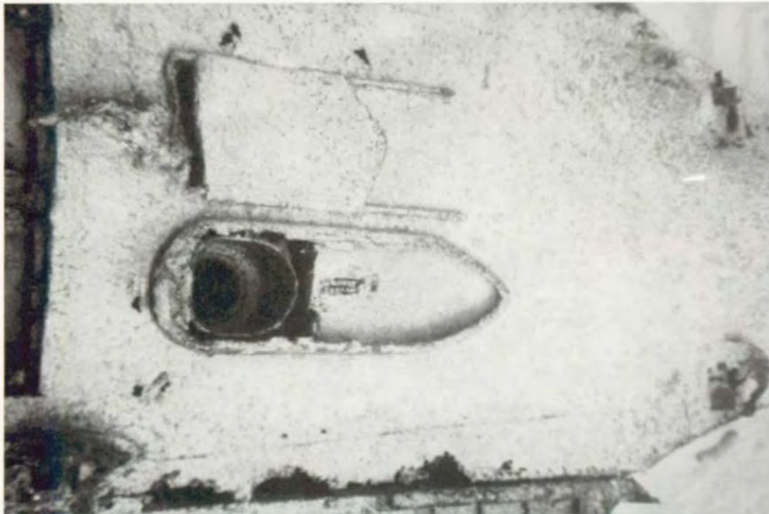
Fig. 11.12. The camera sight hole, bomb racks and external fuel racks are visible on the remains of this Jake float plane lost in Saipan Lagoon. (Photo by William Cooper)
