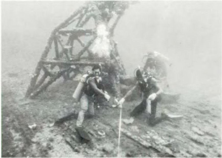
Fig. 9.134. Bikinian divers working with NPS/Navy team on the USS SARATOGA. They are measuring in the location of a "Christmas tree," a specially designed tower for holding blast gauges and other test instruments. (NPS photo by Larry Murphy)
