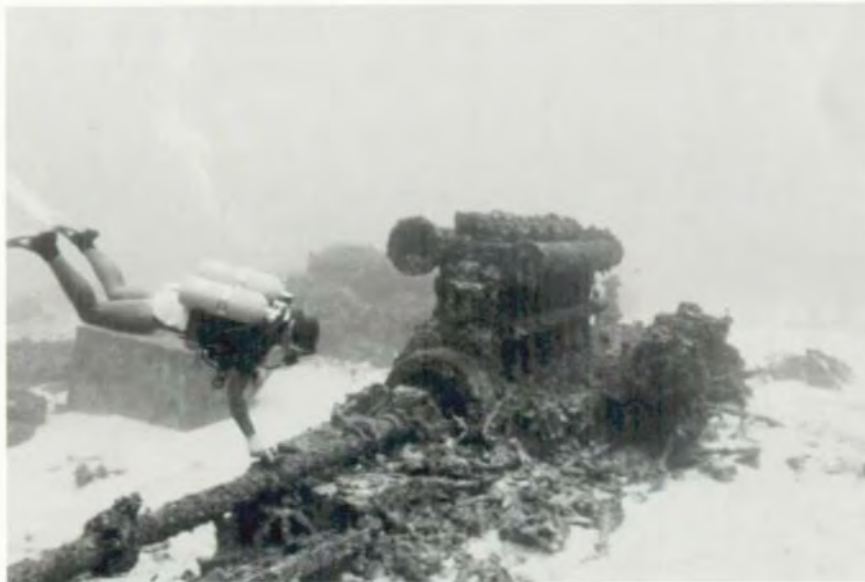
Fig. 9.26. The diesel engine from auxiliary submarine chaser site Number 2 at Coral Gardens sits upright with its shaft still attached. Note the fuel tank beyond the diver. (Photo by Tim Rock)
