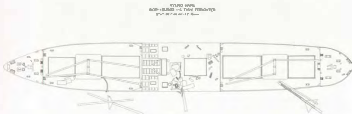
Fig. 9.93. Line drawing of 1C freighter sunk in Belau, March 1944, possibly RYUKO MARU.
