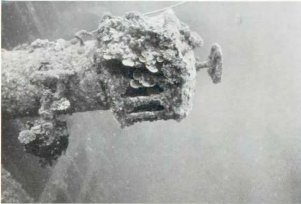
Fig. 9.50. Valve handle, probably for ventilator, on mast cap of TOKAI MARU. (NPS photo by Larry Murphy)
