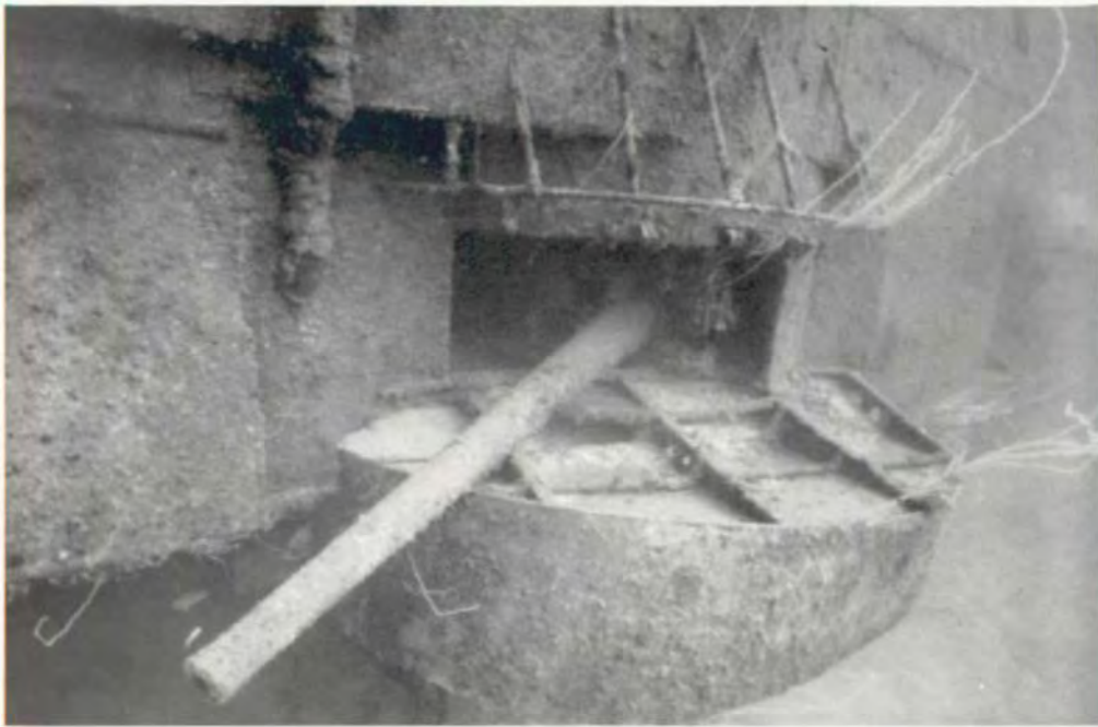
Fig. 9.136. A 5-inch gun protrudes from a forward casemate on the battleship USS ARKANSAS in Bikini Atoll Lagoon. It lies upside down as does Japanese battleship NAGATO close by. (NPS photo by Larry Murphy)
