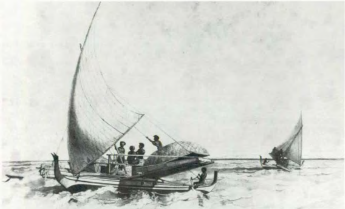
Fig. 4.8. Carolinian proas. The ubiquitous popo as depicted by Admiral Paris has not changed perceptibly for centuries. Still in use, it is lateen-sailed, twin-ended and single-outriggered. These Satawal canoes are exactly like those of Yap, Ulithi and the rest of the west-central Carolines. Source: Paris 1843:II, pl. 107. (Courtesy UCLA Library)
