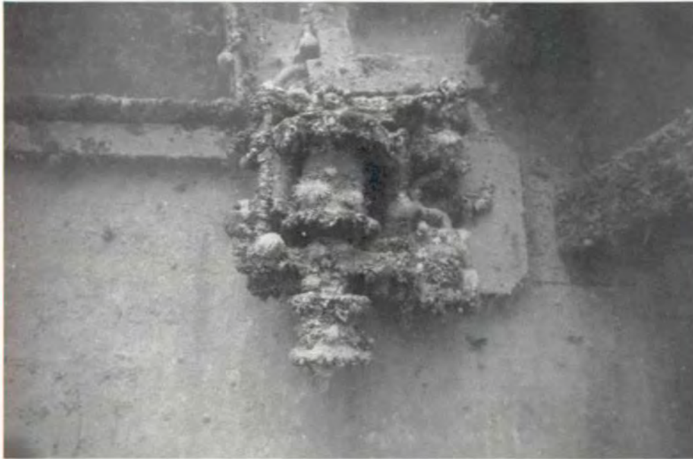
Fig. 9.111. Small cargo winch located at the engine room cargo hatch. (NPS photo by Toni Carrell)
